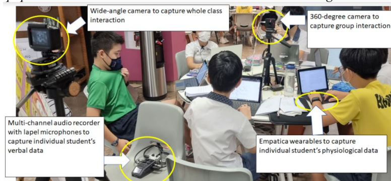
Figure 1 Equipment and sensors used to record multimodal data during the lesson
